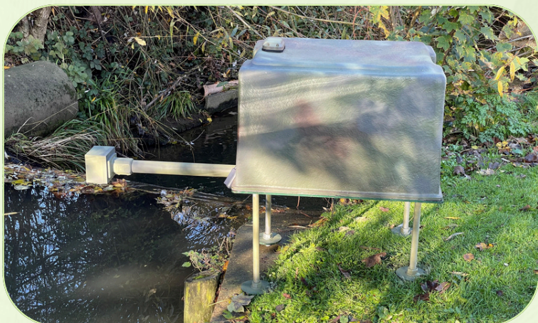
Figure 2. 'Turtle' gauge measuring Pix Brook water level
