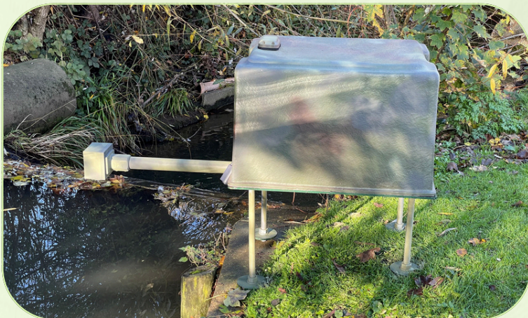
Figure 2. 'Turtle' gauge measuring Pix Brook water level
