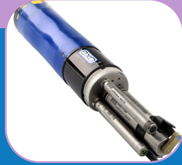
Figure 1: XYLEM YSI EXO-1 - Water Quality Sonde
